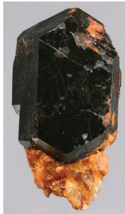
FIGURE 3. Uraninite crystal (1 cm in length) with feldspar from the Swamp Mine, Maine. Uraninite crystals precipitated from magmatic-related fluids typically contain significant quantities of Th, up to about 12 wt% ThO 2 , although U has been greatly enriched in such systems relative to Th compared with crustal igneous source rocks. Photo courtesy of Robert Lauf. Crystal is 1.5 cm tall.
