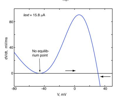
a saddle-node bifurcation. Izhikevich argues that this is a model for the rising phase of an action potential. If the model were suddenly depolarized by such a current, the membrane potential would jump from  $\sim$ -50 mV to  $\sim$ -30 mV (assuming it started at -50 mV).
