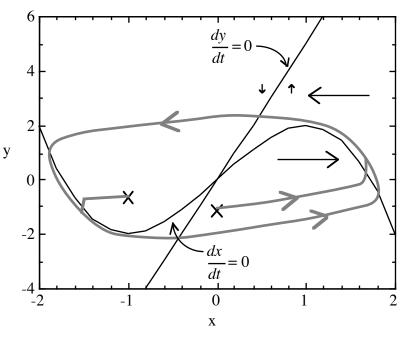
two values, 0.5 and 0.1. In the first case, the difference in time scale of the differential equations is small and the actual trajectories are not well approximated by the assumed trajectories drawn above. In the second case, the trajectories follow the dx/dt=0 nullcline quite closely.
