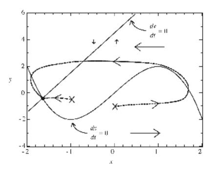
The arrows show the directions of flow in the phase plane relative to the two isoclines. Notice that the x-arrows are much larger than the y-arrows, as is (qualitatively) consistent with the problem statement ( $\varepsilon <<1$ ). The equilibrium point at the intersection of the isoclines occurs at
